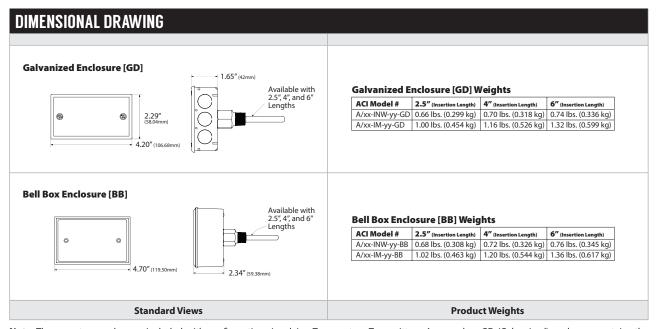
Note: There are two enclosures included with configurations involving Temperature Transmitters. A secondary GD (Galvanized) enclosure contains the transmitter board to protect it from the extreme temperatures exposed to the sensing element
